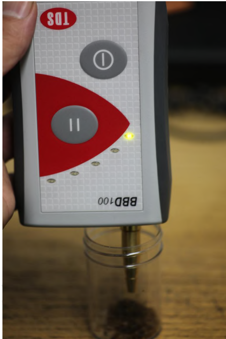
Definitive test showing a failure to detect even the significant number of bedbugs shown in the picture above.
